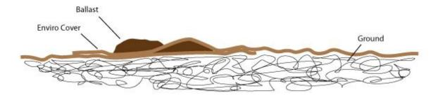
Figure 3 – Cross-section of overlapped film edges with ballasted mounds adjacent to each other in such a way as to provide an effective edge seal.
