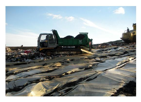
Figure 2 - The EPI Model 800 Deployer at Puente Hills, a track mounted self-propelled film and ballast deploying device with excellent capability for efficient movement and coverage.
