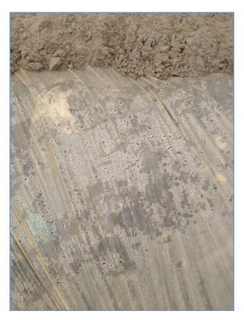
Enviro™ Cover's impermeable barrier blocks gas and odors that rise with condensation as shown on the underside
