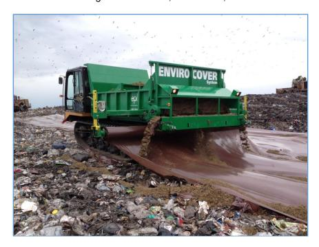
The Model 800 Deployer, deploying plastic film while it lays down soil ballast strips for anchoring the film and sealing the overlapped panels providing complete and confirming coverage
